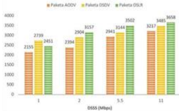
Fig. 8: The dependence of the number of received packets from the DSSS change
